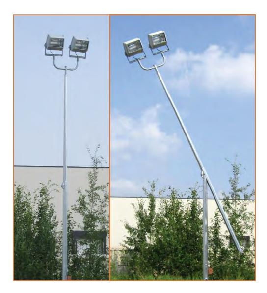
Built to AASHTO standards, the Tiltable Steel Pole is fabricated from structural steel and hot-dipped galvanized for increased durability. In addition, the octagonal shape provides minimal resistance to the wind while rigidly supporting airfield equipment. The pole can be left bare or can be painted orange and white per Transport Canada, ICAO, and FAA obstruction marking requirements.
